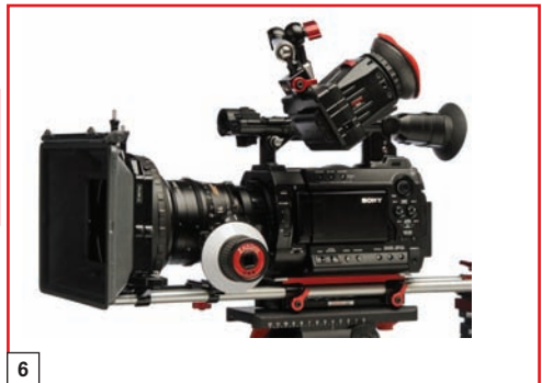
Ενδιαφέρον studio-configuration της F3 με matte-box, follow-focus, base-plates & orientable viewfinder
