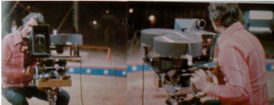
Unidentified geared head taking a 70mm camera on its side for vertical recording and future vertical display.
