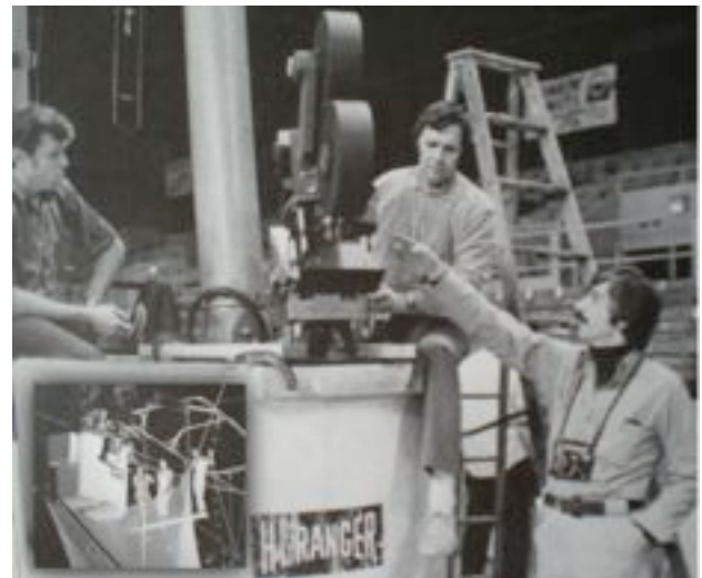
Geared head mounted to planks of wood, riding up in a bucket for some high-up shots of trapeze performers (aka cherry picker, condor, etc.)
