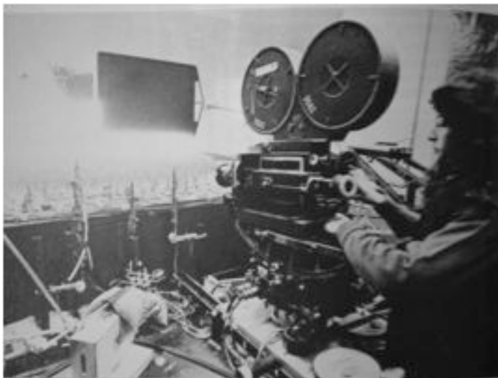
This geared head is electronically driven via motion control. Miniature cityscape from Blade Runner , 1981.
