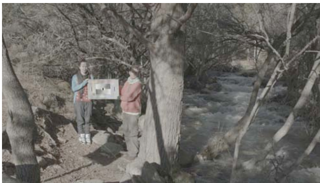
24mm lens. T 6.3. LogC800. 5600°K. 25fps. Obt 180°. ND 0.9 filter. Original of Camera.
